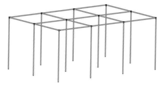
N.B. You should assemble the roof fittings with the grub screws facing down to make it easier to adjust them when the roof is complete. This is the opposite to how they were assembled on the ground so you will need to flip any partially assembled pieces the other way around.
